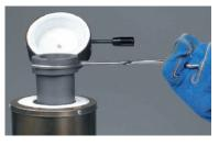
Beginning with small pieces, slowly add metal to the crucible, fill the crucible only to 1/4 – 1/3 of its capacity at first. Once that is melted, add more metal until you have the amount needed for your casting.
