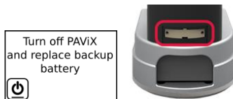
Figure 37: Low battery warning and battery housing for the height measuring function (CR2032)
