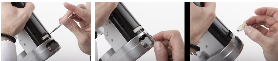
Figure 29: CR2032 battery holder
