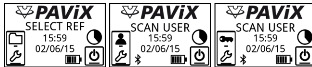
Figure 51: Home screen without a scanner then in User or Expert mode with a connected scanner
