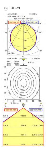
light source LED work equipment electronic transformer connected load 100-240 V, 50/60 Hz; secondary 24 V, DC power consumption env. 30 W luminous flux approx. 2.000 lm luminous efficiency approx. 77 lm/W light type/-color cold white colour temperatur approx. 5.000 K color rendering index CRI > 90; R9 > 50 light distribution direct direct ratio approx. 100 % beam angle 110° chromaticity tolerance LED < 3 SDCM
